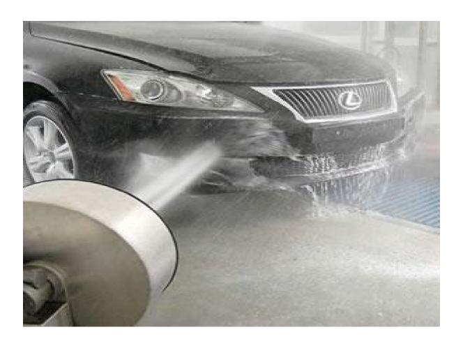
• Tire spinner, high pressure nozzles angled specifically to clean wheels and tires.
