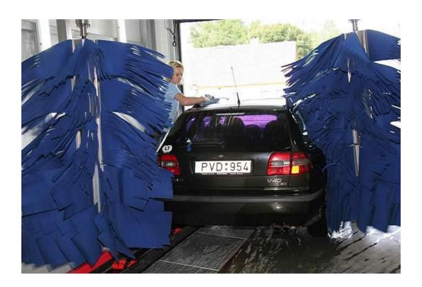
• An attendant (or signage) manually drying a car after conveyorized automatic washing.
